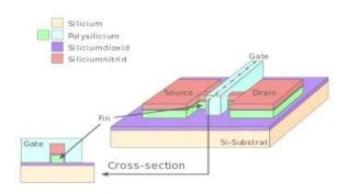
Fig: 2 Schematic diagram of FinFet
